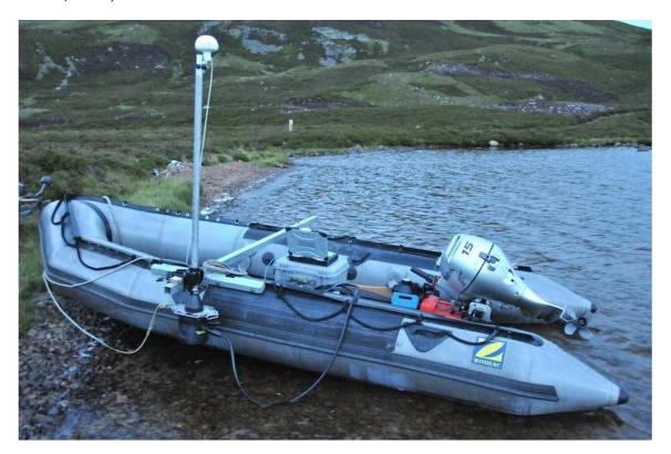
Figure 8. A hydroacoustics system deployed on a 4.8 m RIB. Sound is projected and recorded by a transducer mounted on a vertical pole to the side of the vessel, with a GPS receiver mounted at its top to provide positional information. The system's surface unit is visible as a grey case in the centre of the vessel, with a controlling laptop computer on top of it. The system is powered by a single 12 V battery visible in a blue casing towards the stern of the vessel. © lan Winfield.
