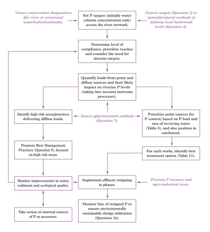
Figure 9. Process diagram for developing a phosphorus control strategy within a river catchment, with links to information in this document.
