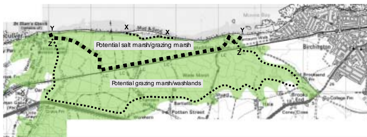
Figure 2.8 Main 'set-back' lines for habitat recreation and creation within a flood risk area
