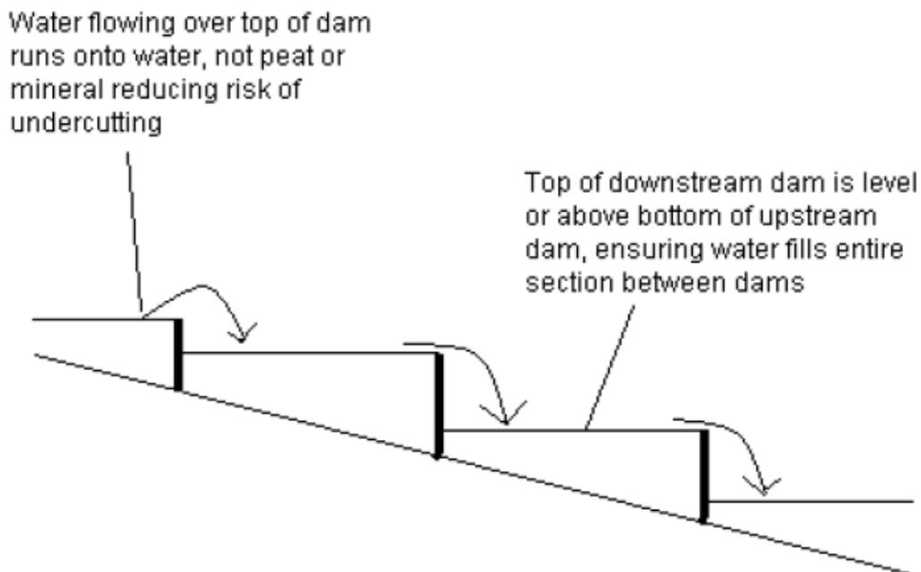
Figure 3-33: Spacing of Dams in a Gully (from Evans *et al.*, 2005)
