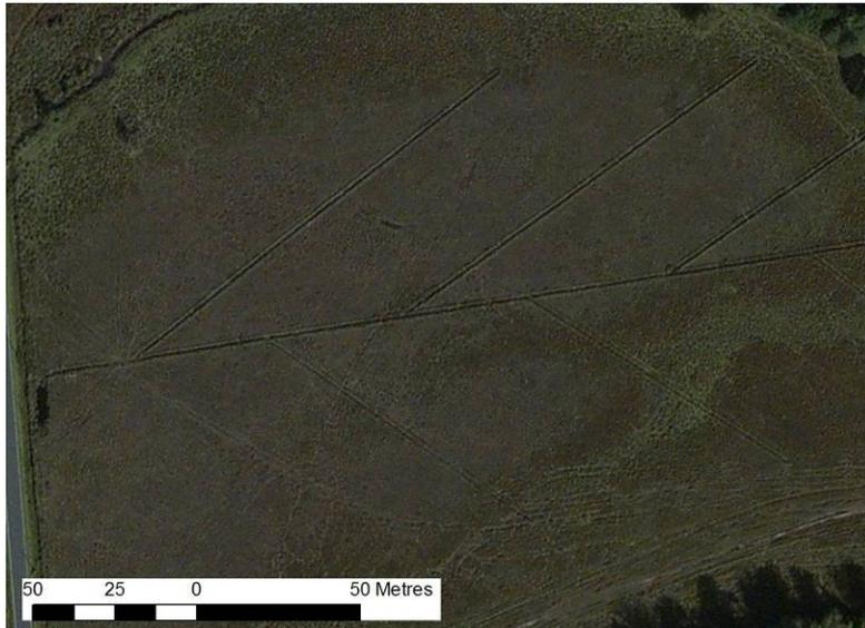
**Figure 3-15: Aerial photography of herringbone drainage south of Dibden Bottom**
