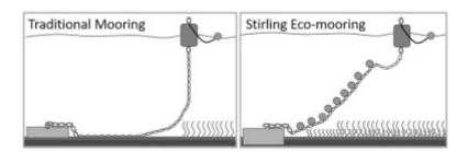
Figure A 1: Diagram showing a traditional swing mooring (left) and the National Marine Aquarium's Stirling Ecomooring (right). The Eco-mooring has buoys along the riser chain keeping it off the seabed and double the tonnage of a standard ground weight. Image adapted from one provided by the National Marine Aquarium. Source: Parry-Wilson and others, 2019. Crown Copyright © 2019 Published by Elsevier Ltd. All rights reserved. Reproduced with permission.
