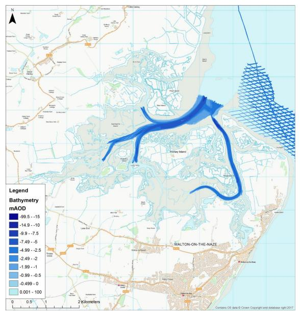
Figure 4.3. Environment Agency multibeam echosounder data in Hamford Water (<u>http://environment.data.gov.uk/ds/survey/index.jsp#/survey</u>)
