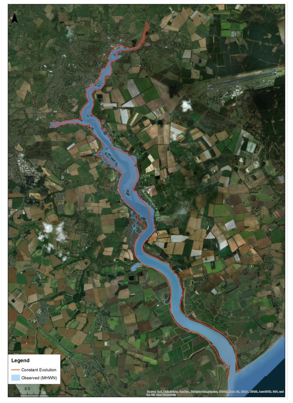
Figure 3.9. Comparison of predicted equilibrium widths with observed widths in the Deben Estuary (aerial photograph background)
