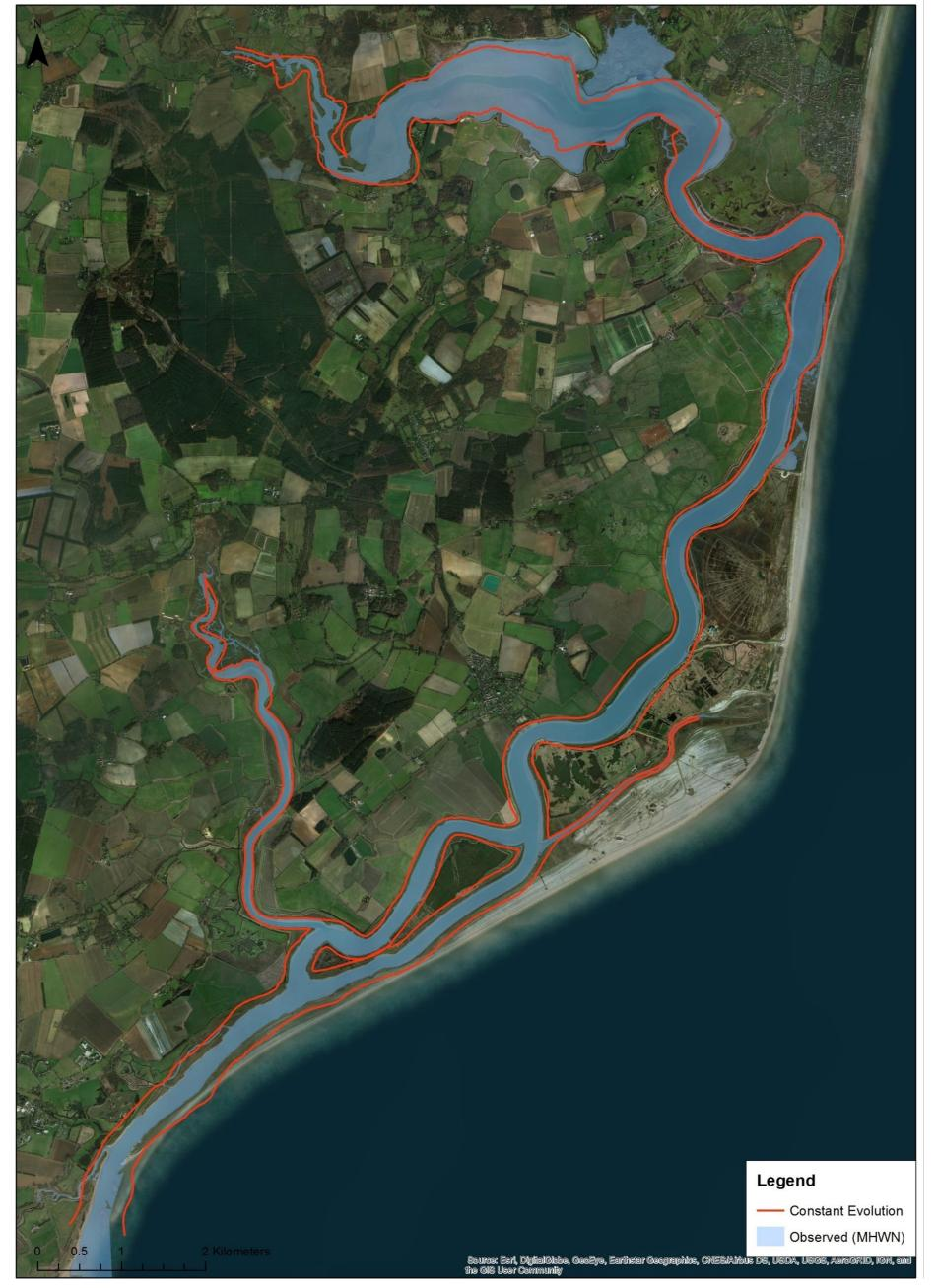
Figure 2.9. Comparison of predicted equilibrium widths with observed widths in the Alde-Ore Estuary (aerial photograph background)
