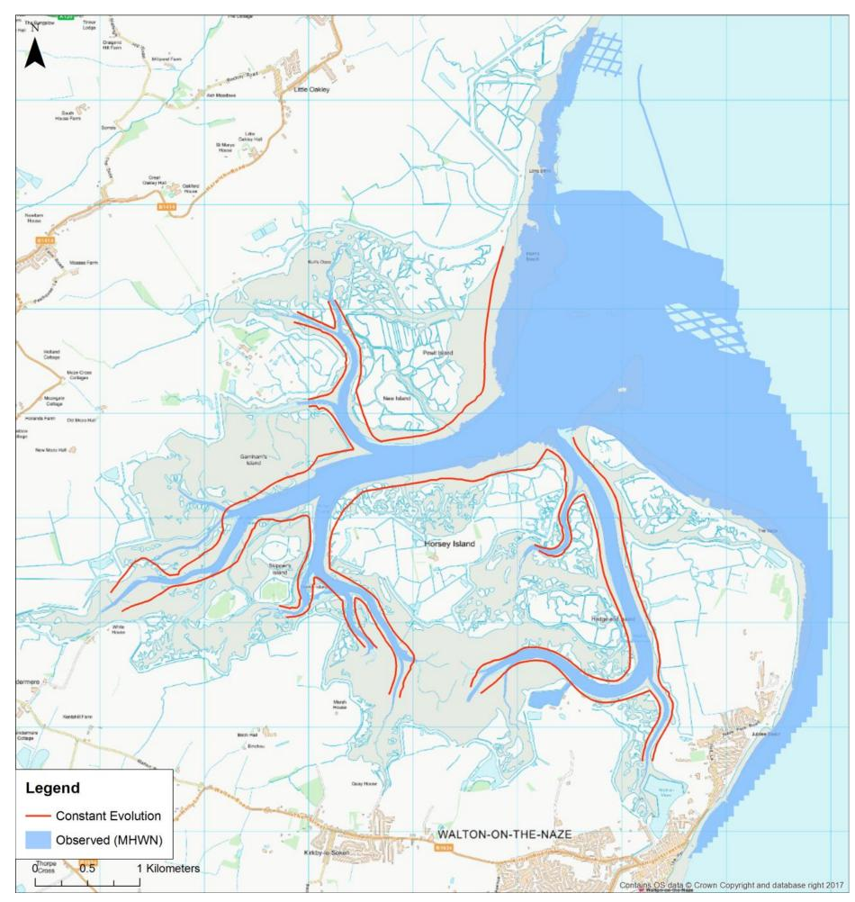
Figure 4.9. Comparison of predicted equilibrium widths with observed widths in Hamford Water (map background)
