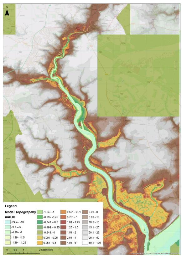
Figure 3.5. Combined LiDAR, multibeam echosounder and interpolated bathymetry in the Deben Estuary
