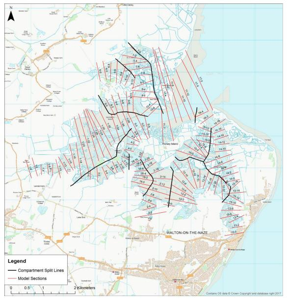
Figure 4.8. Location of sections in Hamford Water. The black lines are the locations of the 'tidal watersheds' driving the tidal prism along the adjacent channels
