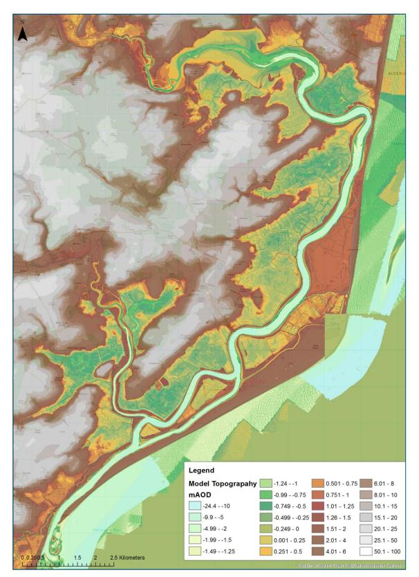
Figure 2.5. Combined LiDAR, multibeam echosounder and interpolated bathymetry in the Alde-Ore Estuary and Butley Estuary
