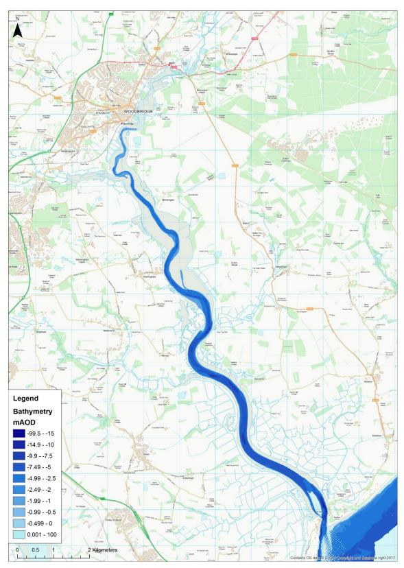
Figure 3.3. Environment Agency multibeam bathymetry data in the Deben Estuary (http://environment.data.gov.uk/ds/survey/index.jsp#/survey)
