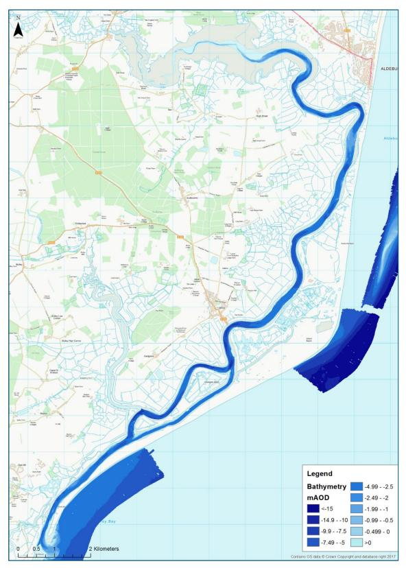
Figure 2.3. Environment Agency multibeam bathymetry data in the Alde-Ore Estuary (http://environment.data.gov.uk/ds/survey/index.jsp#/survey)
