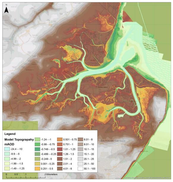
Figure 4.6. Combined LiDAR, multibeam echosounder and single beam echosounder data in Hamford Water
