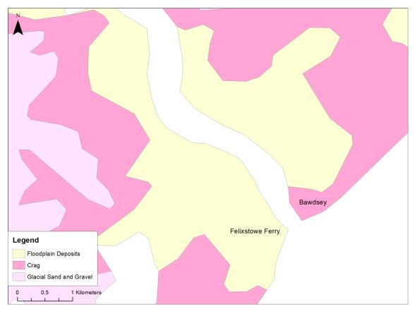
Figure 3.10. Geological constraints at Bawdsey at the mouth of the Deben Estuary. Map is based on 1:625,000 scale data from the British Geological Survey
