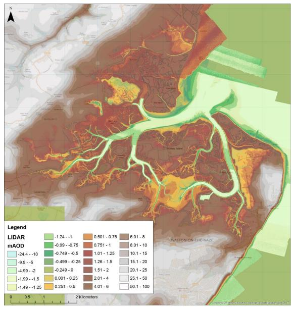
Figure 4.2. Environment Agency LiDAR data in Hamford Water (<u>http://environment.data.gov.uk/ds/survey/index.jsp#/survey</u>)
