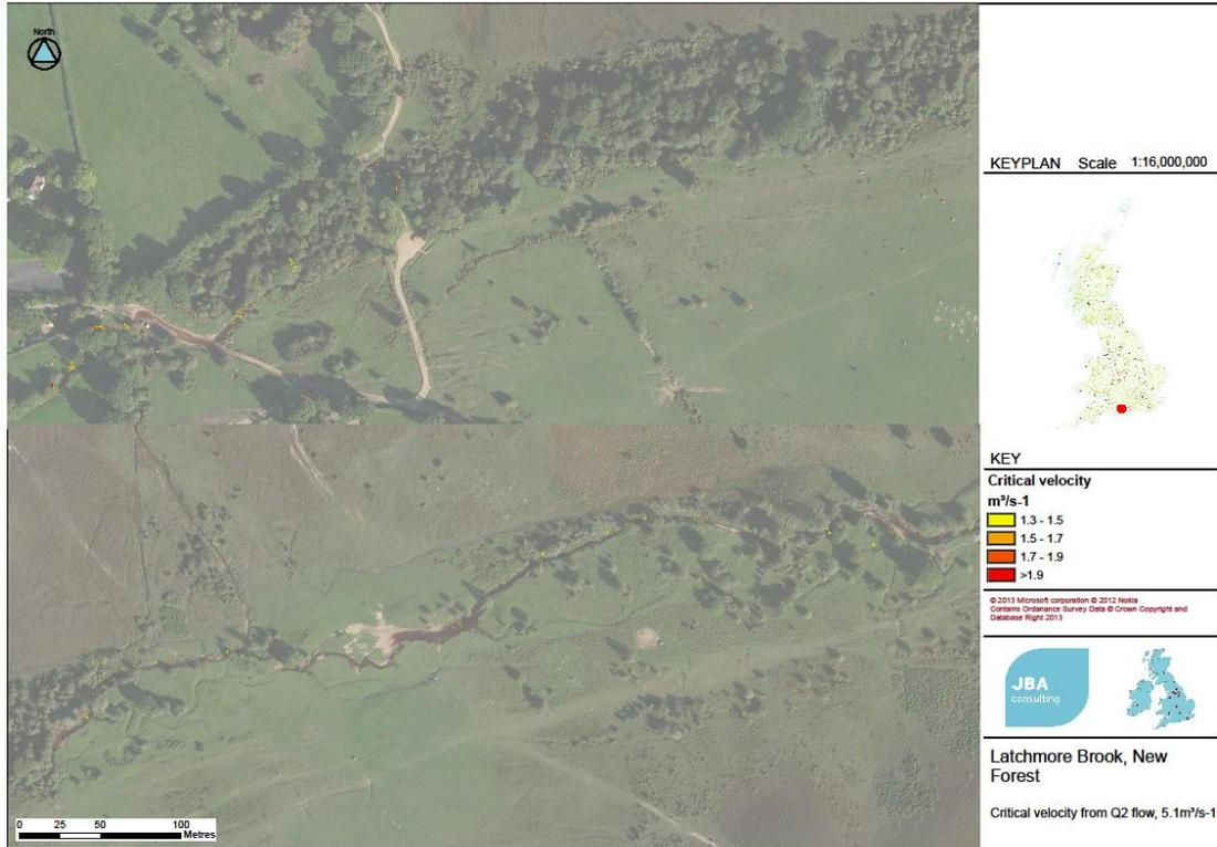
Figure 4-13b: Plot of critical velocity sites for the 2 year return period flow along the naturalising anastomosed Latchmore Brook
