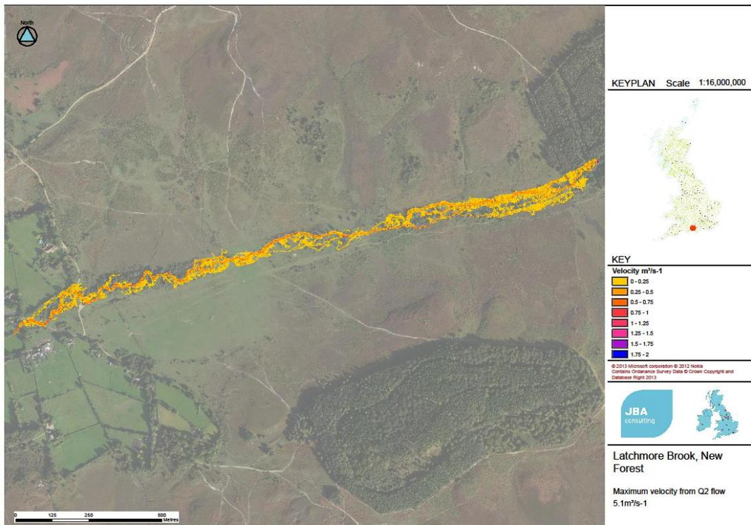
Figure 4-5a: Plot of critical velocity sites for the 2 year return period flow along the current Latchmore Brook
