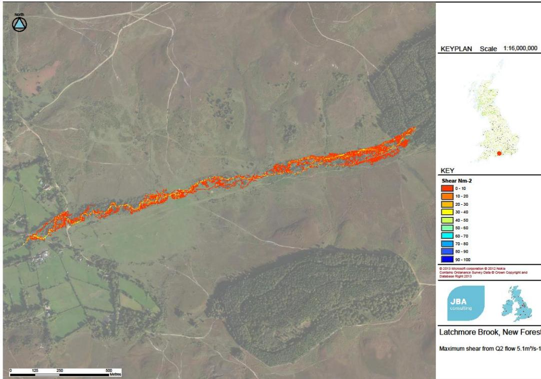
Figure 4-7: Plot of critical shear stress sites for the 2 year return period flow along the current Latchmore Brook
