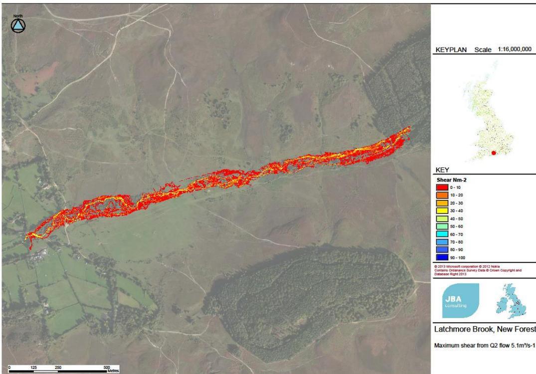
Figure 4-15: Plot of critical shear stress sites for the 2 year return period flow along the naturalising anastomosed Latchmore Brook
