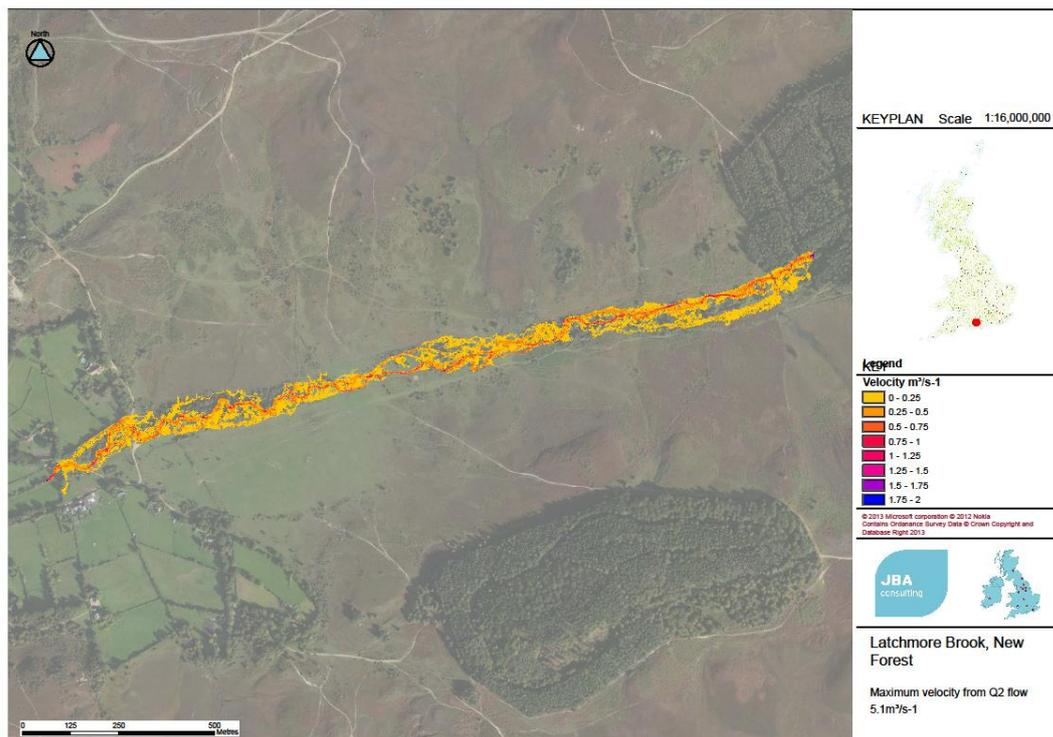
Figure 4-9a: Plot of critical velocity sites for the 2 year return period flow along the re-meandered Latchmore Brook
