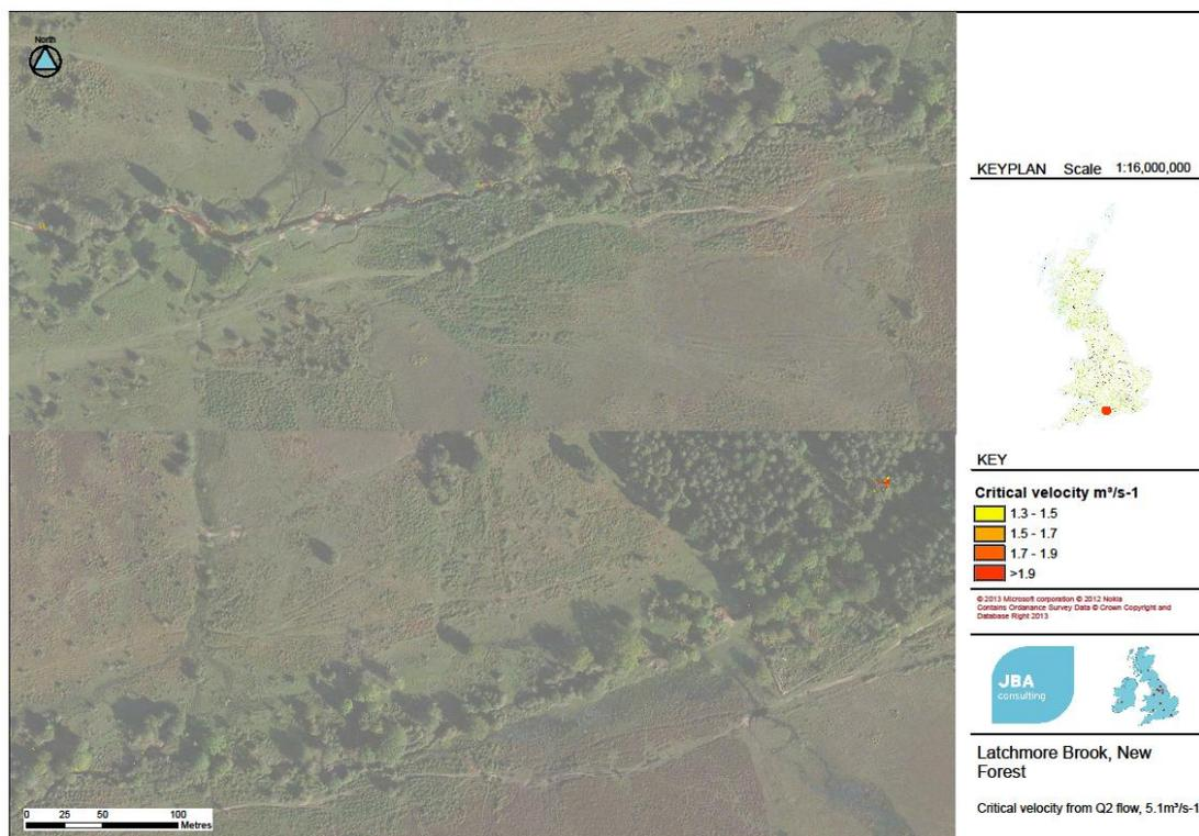
Figure 4-10: Plot of shear stress distribution for the 2 year return period flow along the re-meandered Latchmore Brook
