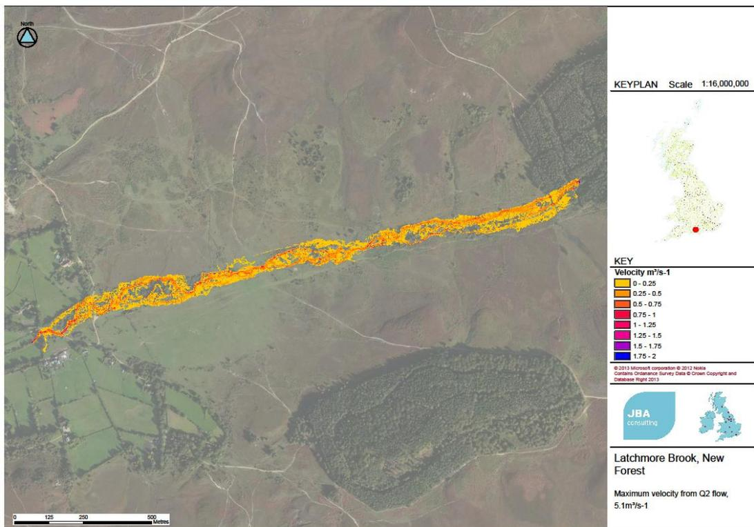
Figure 4-13a: Plot of critical velocity sites for the 2 year return period flow along the naturalising anastomosed Latchmore Brook
