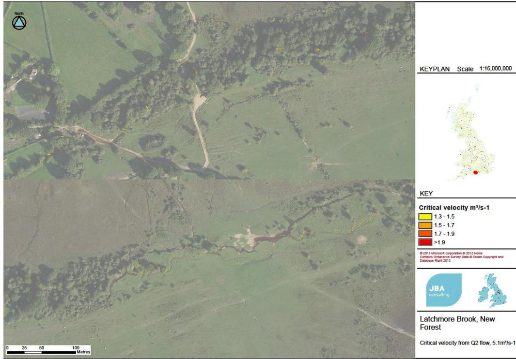
Figure 4-9b: Plot of critical velocity sites for the 2 year return period flow along the re-meandered Latchmore Brook
