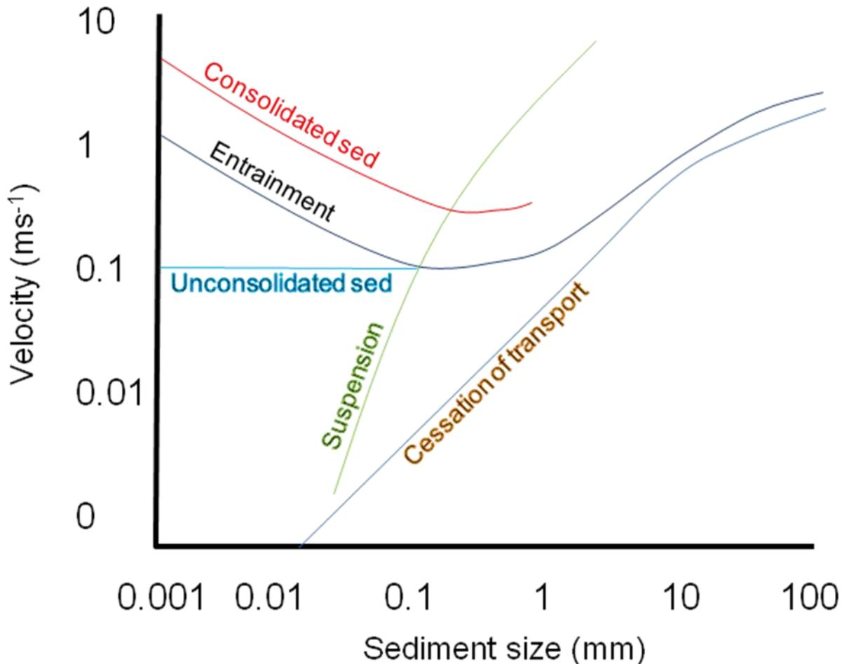
With respect to unconsolidated sediments the critical threshold for movement ( $\tau_{cr}$ ) may be calculated from the Shields entrainment function:
