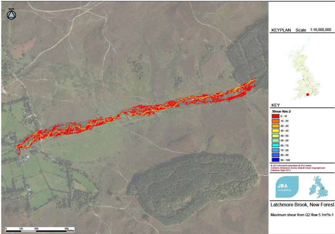
Figure 4-11: Plot of critical shear stress sites for the 2 year return period flow along the re-meandered Latchmore Brook
