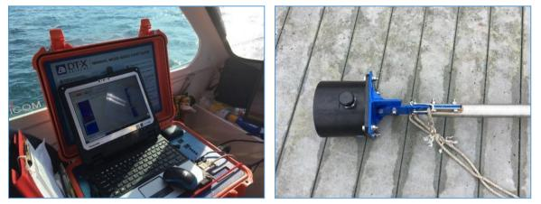
**Figure 3**. The BioSonics DT-X Extreme surface unit (left) and pole-mounted 200 kHz transducer (right).
