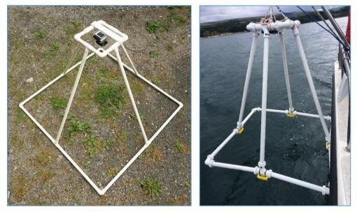
Figure 2. The 1 m<sup>2</sup> photo-quadrat with GoPro camera mounted directly above the quadrat
