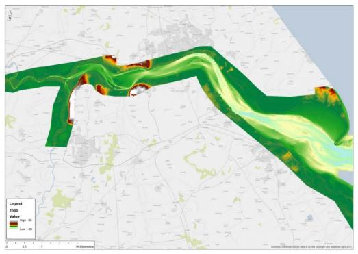
Figure 4.1. Humber Estuary bathymetry created by combining interpolated echosounder data with LiDAR data (see Figure 3.1)
