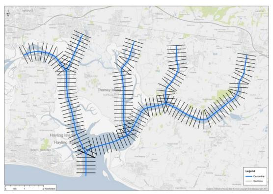
Figure 4.7. Automatic positioning of sections in Chichester Harbour at the spacing prescribed by the user (200m in this case)
