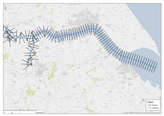
Figure 4.6. Automatic positioning of sections in the Humber Estuary at a spacing prescribed by the user (1km in this case)
