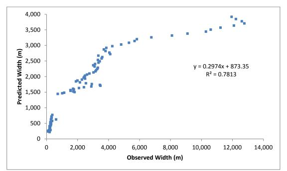
Figure 5.11. Comparison of observed and predicted widths in the Humber Estuary using the regime equation for Group C estuaries and the Lacey equation with an input particle size of 0.2mm.
