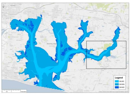
Figure 4.4. Tidal datum surfaces in Chichester Harbour. MHWS = Mean High Water Spring. MHWN = Mean High Water Neap. MLWS = Mean Low Water Spring. Box is enlarged in Figure 4.5.
