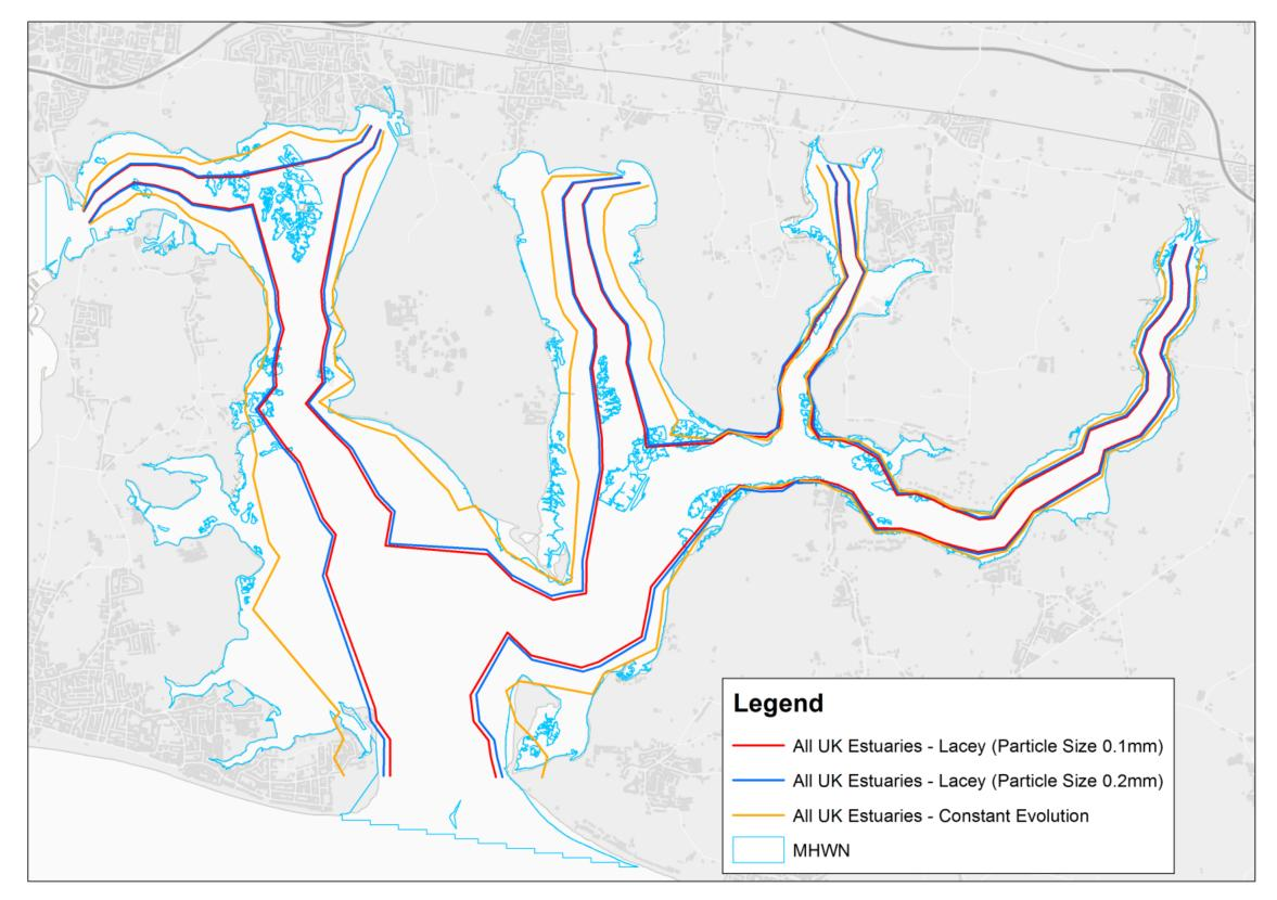
Figure 5.4. Comparison of observed and predicted widths in Chichester Harbour using the regime equation for all United Kingdom estuaries combined with 1. particle size of 0.1mm in the Lacey (1930) equation (red), 2. particle size of 0.2mm in the Lacey (1930) equation (blue), and 3. the 'constant evolution' relationship (orange)
