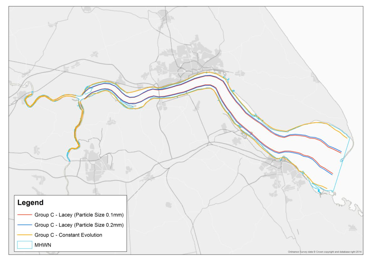
Figure 5.2. Comparison of observed and predicted widths in the Humber Estuary using the regime equation for United Kingdom estuaries Group C combined with 1. particle size of 0.1mm in the Lacey (1930) equation (red), 2. particle size of 0.2mm in the Lacey (1930) equation (blue), and 3. the 'constant evolution' relationship (orange)
