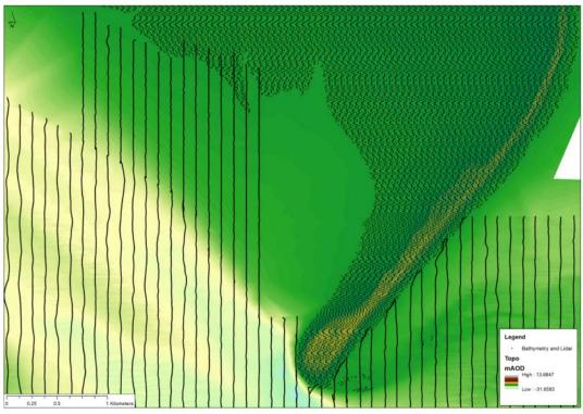
Figure 3.1. Echosounder transects and LiDAR data for the Humber Estuary collected in 2005 by Associated British Ports
