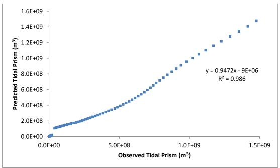
Figure 5.8. Comparison of observed and predicted tidal prisms in the Humber Estuary
