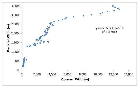
Figure 5.10. Comparison of observed and predicted widths in the Humber Estuary using the regime equation for Group C estuaries and the Lacey equation with an input particle size of 0.1mm.
