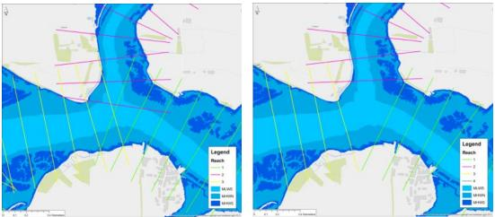
Figure 4.9. Example of when to manually move or remove automated sections that overlap at channel confluences
