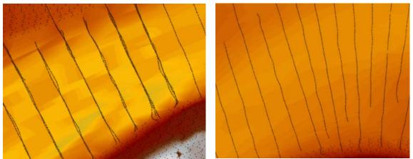
Figure 3.5. Interpolated multiple overlapping transects in the Humber Estuary (left) compared to interpolated single transects (right).
