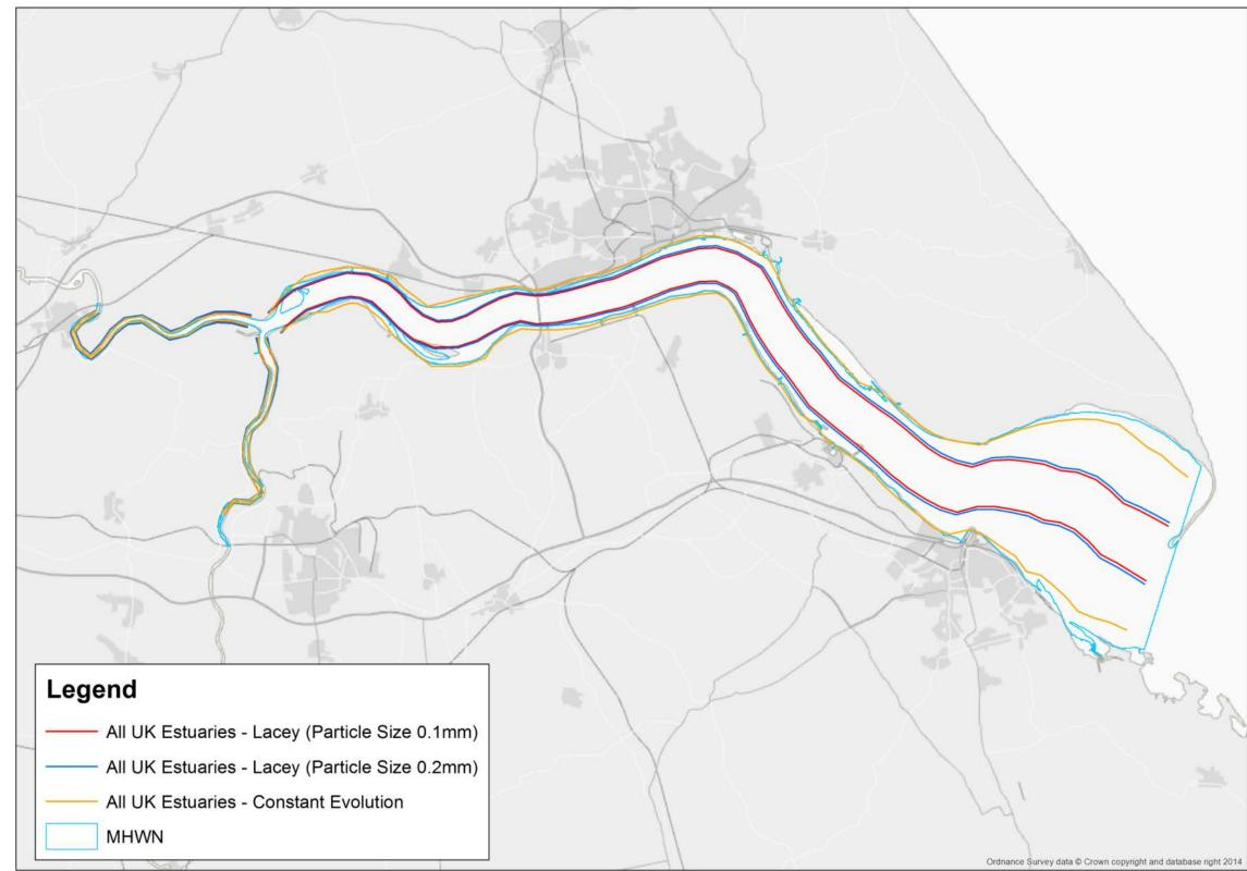
Figure 5.1. Comparison of observed and predicted widths in the Humber Estuary using the regime equation for all United Kingdom estuaries combined with 1. particle size of 0.1mm in the Lacey (1930) equation (red), 2. particle size of 0.2mm in the Lacey (1930) equation (blue), and 3. the 'constant evolution' relationship (orange)
