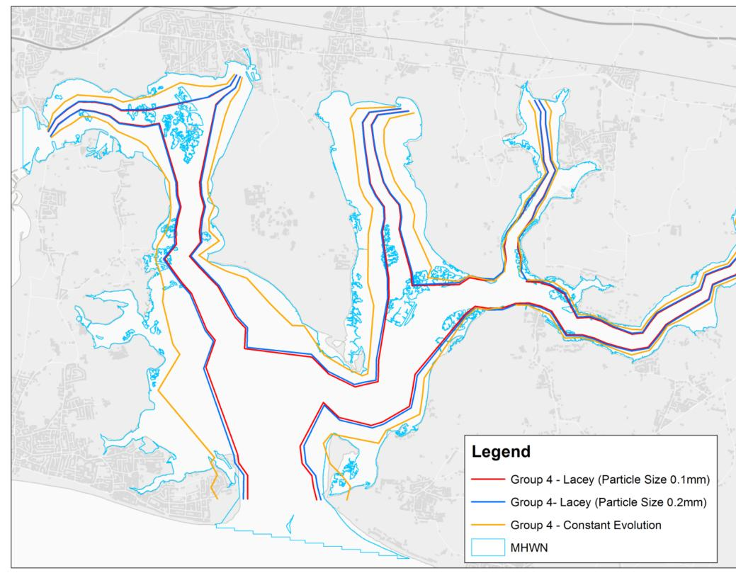
Figure 5.6. Comparison of observed and predicted widths in Chichester Harbour using the regime equation for United Kingdom estuaries Group 4 combined with 1. particle size of 0.1mm in the Lacey (1930) equation (red), 2. particle size of 0.2mm in the Lacey (1930) equation (blue), and 3. the 'constant evolution' relationship (orange)
