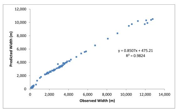
Figure 5.12. Comparison of observed and predicted widths in the Humber Estuary using the regime equation for Group C estuaries and the 'constant evolution' relationship.
