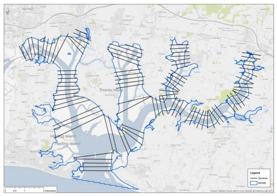
Figure 4.11. Final position of sections in Chichester Harbour after automatic positioning followed by manual manipulation
