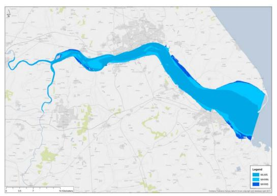
Figure 4.3. Tidal datum surfaces in the Humber Estuary. MHWS = Mean High Water Spring. MHWN = Mean High Water Neap. MLWS = Mean Low Water Spring.
