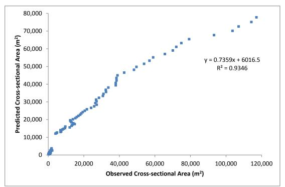
Figure 5.9. Comparison of observed and predicted cross-sectional areas in the Humber Estuary using the regime equation for Group C estuaries
