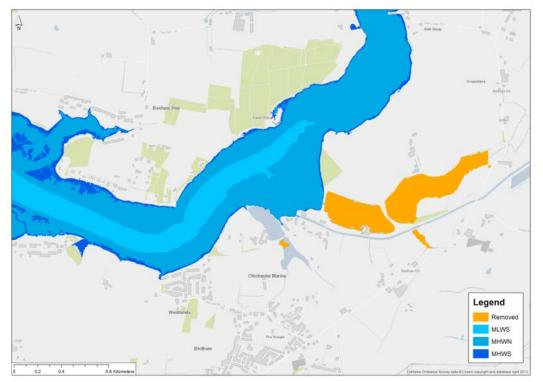
Figure 4.5. An example of superfluous datum surfaces (in orange) in Chichester Harbour. Location is shown in Figure 4.4. These surfaces were created in the GIS but are not part of the channel that is affected by the tidal prism, so they should be removed.
