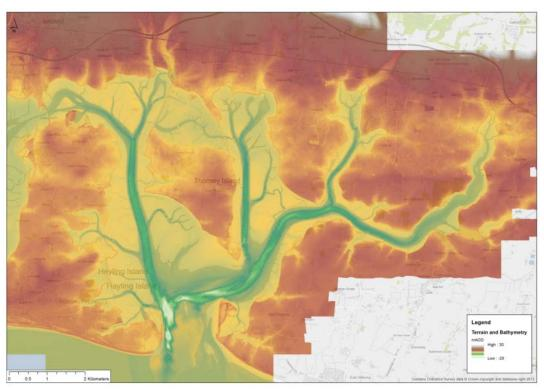
Figure 4.2. Chichester Harbour bathymetry created by combining interpolated echosounder data with LiDAR data (see Figure 3.2).
