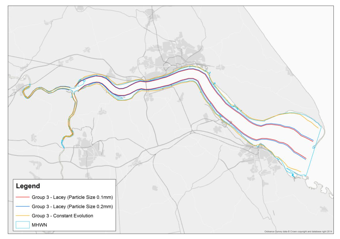
Figure 5.3. Comparison of observed and predicted widths in the Humber Estuary using the regime equation for United Kingdom estuaries Group 3 combined with 1. particle size of 0.1mm in the Lacey (1930) equation (red), 2. particle size of 0.2mm in the Lacey (1930) equation (blue), and 3. the 'constant evolution' relationship (orange)
