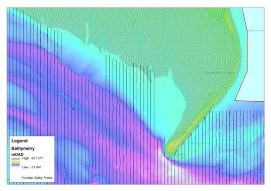
Figure 3.4. Gaps in the Humber Estuary bathymetry data
