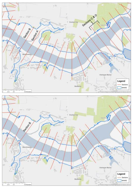
Figure 4.8. Examples of when to manually remove automated sections that cut across both the main channel and a tributary channel
