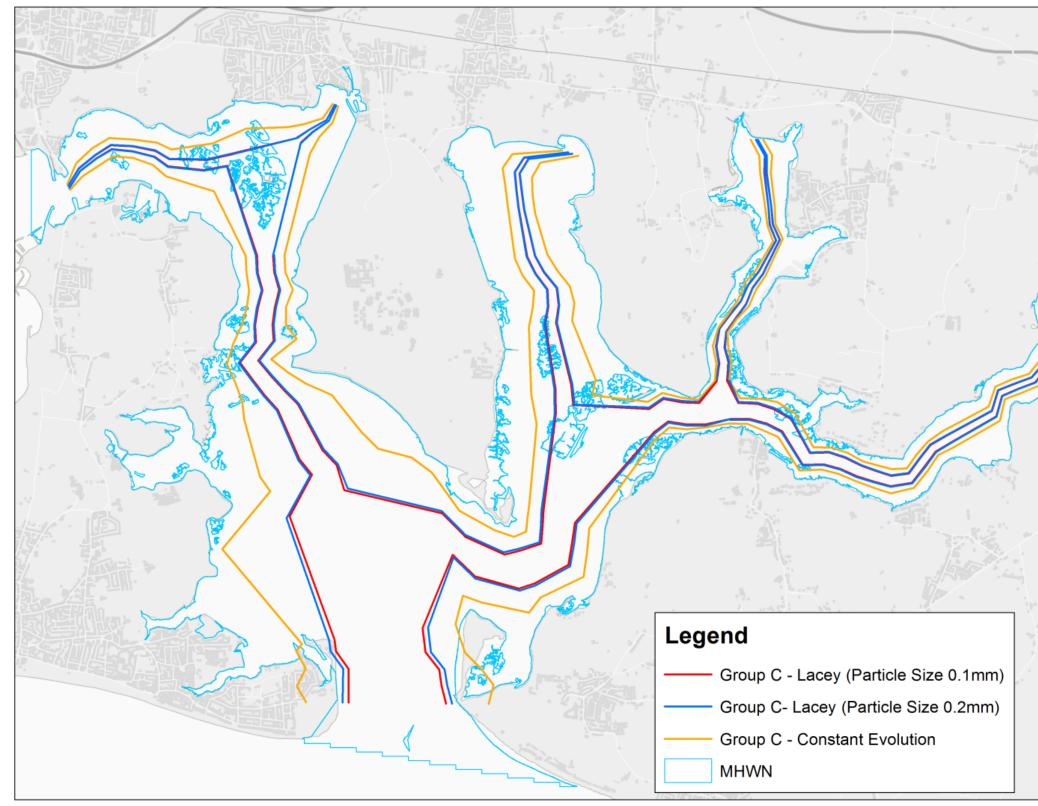
Figure 5.5. Comparison of observed and predicted widths in Chichester Harbour using the regime equation for United Kingdom estuaries Group C combined with 1. particle size of 0.1mm in the Lacey (1930) equation (red), 2. particle size of 0.2mm in the Lacey (1930) equation (blue), and 3. the 'constant evolution' relationship (orange)
