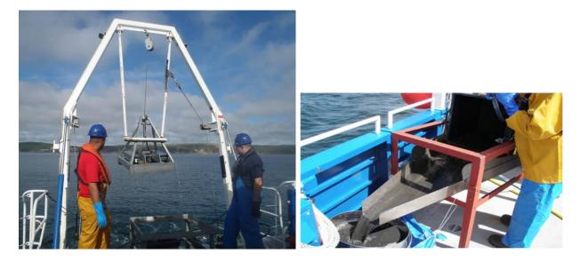
Figure 5. Mini-Hamon Grab (left), and equipment for sieving benthic fauna samples (right).
