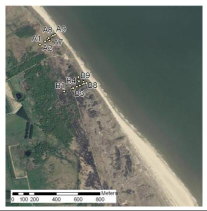
Figure 5. Dipwell monitoring network in the north of the site. Refer to Figure 2 for the location this in the dune system. © NERC (CEH) 2013, © Next Perspectives.
