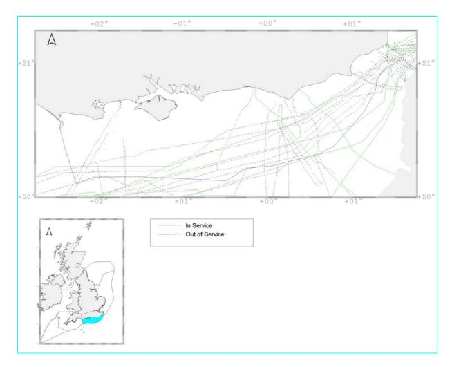
**Figure 6.8** Map of submarine cables passing through the Eastern Channel Natural Area (data provided by Global Marine Systems).
