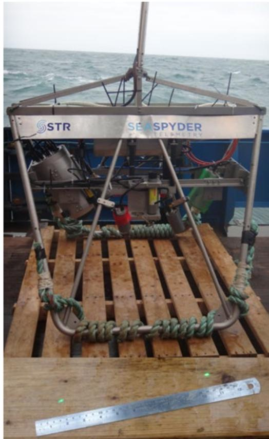
Figure 5. Drop Camera video and still imaging system.
