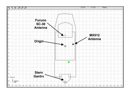
Trimble® HYDROpro<sup>™</sup> vessel editor screen showing survey equipment offsets from the origin (Environment Agency Estuarine and Coastal Monitoring & Assessment Service).
