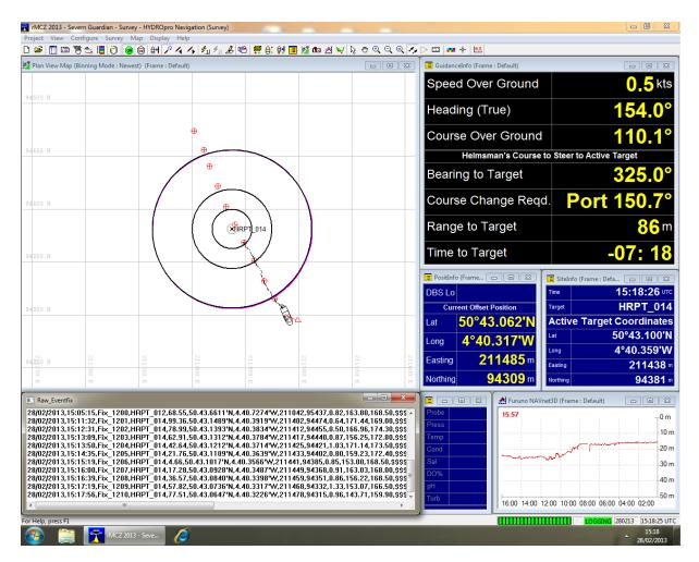
Trimble® HYDRO*pro*<sup>™</sup> software screen grab displaying real-time navigation and survey data acquisition for a MCZ drop camera survey line.
