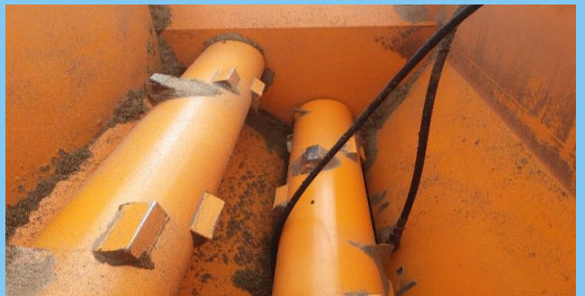
Twin auger 'FLINK bedder' which prevents 'bridging' of the fibre in the machine
