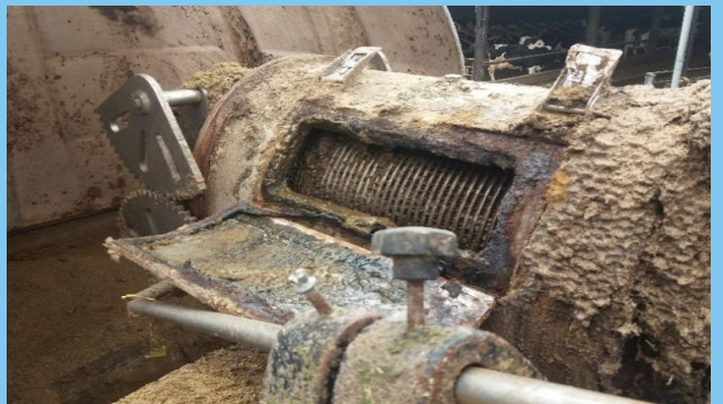
The hard working EYS separator has been in operation for almost 7 years and only had one replacement screen in that time
