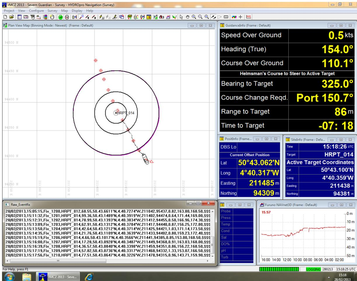
Trimble® HYDROpro™ software screen grab displaying real-time navigation and survey data acquisition for a MCZ drop camera survey line.
