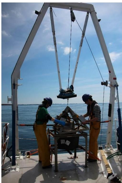
Figure 8. Day grab being deployed from the stern of the vessel.
