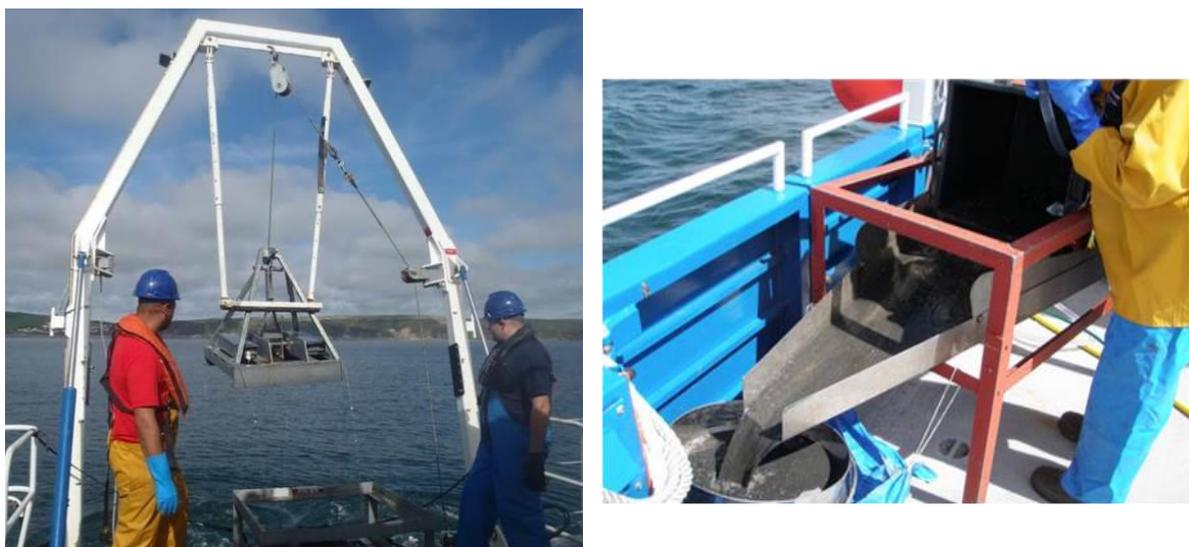
Figure 7. Mini-Hamon grab (left), and equipment for sieving benthic faunal samples (right)
