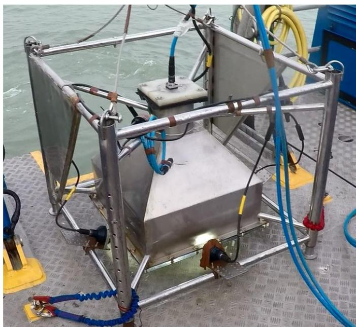
Figure 6. Seastar Survey Ltd. video camera system with freshwater lens.
