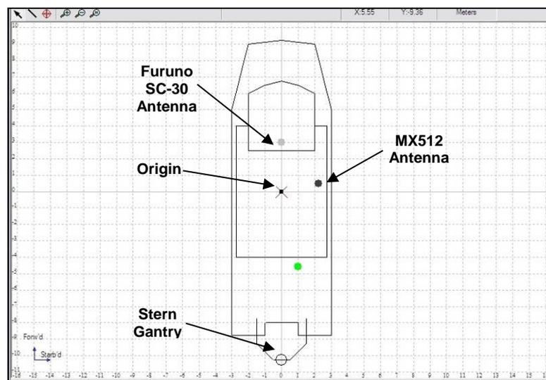
**Trimble® HYDROpro™ vessel editor screen showing survey equipment offsets from the origin
