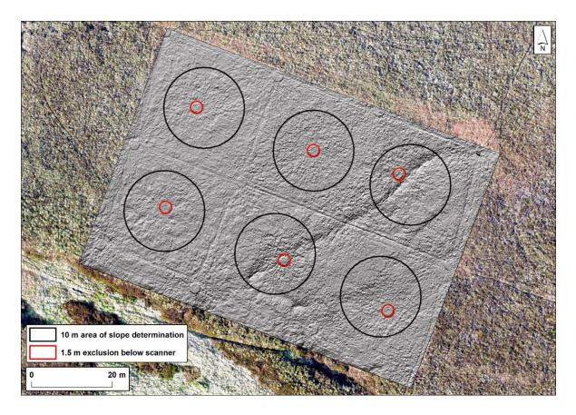
**Figure 22** DTM derived from TLS survey for block D showing area assessed for plot level slope analysis (note the visible depressions in the peat surface created by persistent footfall since 1954, particularly around edges of plots and along the fence lines).
