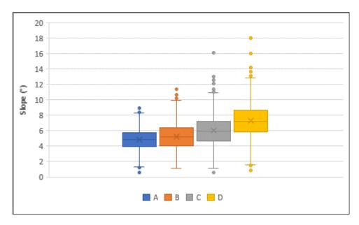
**Figure 20** Slope of the terrain across experimental blocks on Hard Hill derived from airborne Lidar (DTM).
