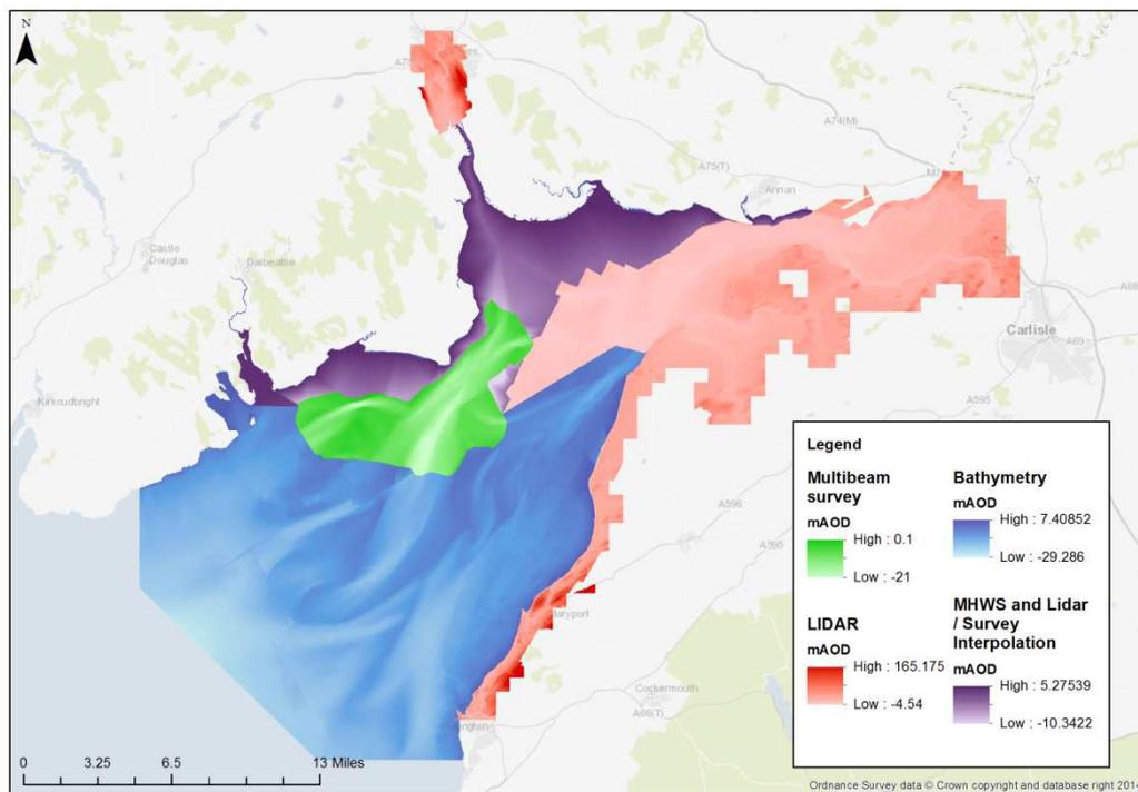
Figure 4.5. Datasets used to create the final bathymetry in the Solway Firth
