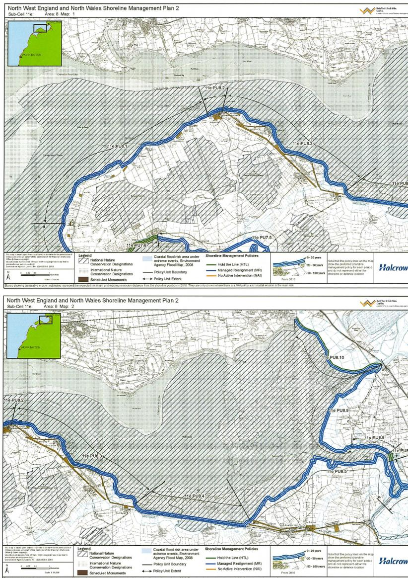
**Figure 4.13. Location of potential managed realignment (blue lines) along the inner Solway Firth (English side) (Halcrow, 2010)**
