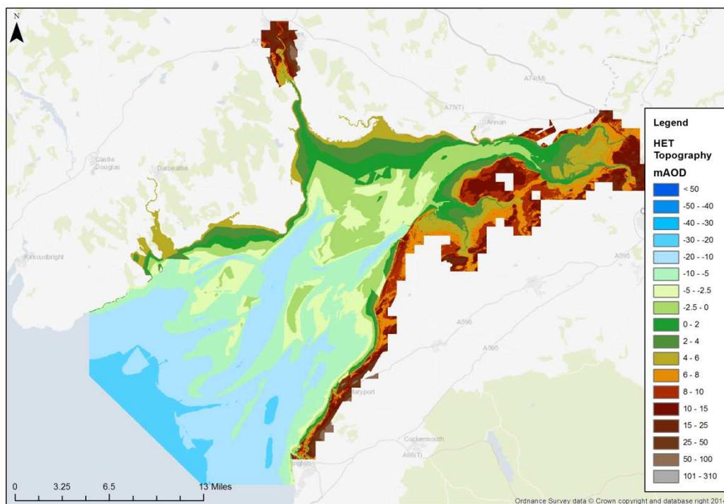
Figure 4.6. Solway Firth bathymetry created by combining all datasets (in OD)
