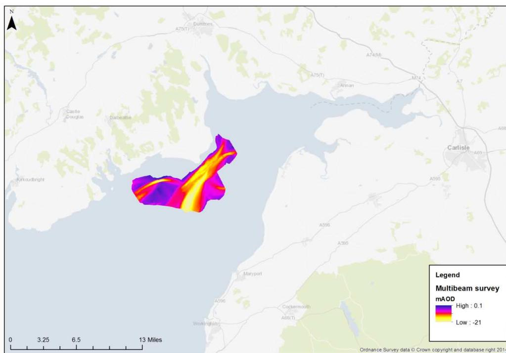
**Figure 4.3. Multibeam bathymetry data in part of the Solway Firth**
