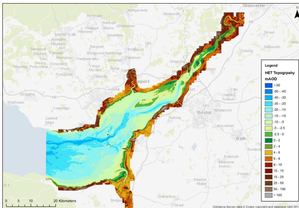
**Figure 3.3. Severn Estuary bathymetry created by combining Admiralty Chart data with LiDAR data (in OD)**
