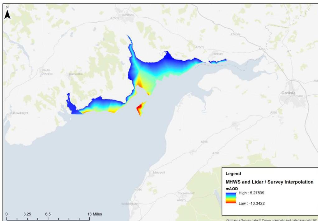
**Figure 4.4. Artificially created bathymetry data in part of the Solway Firth**
