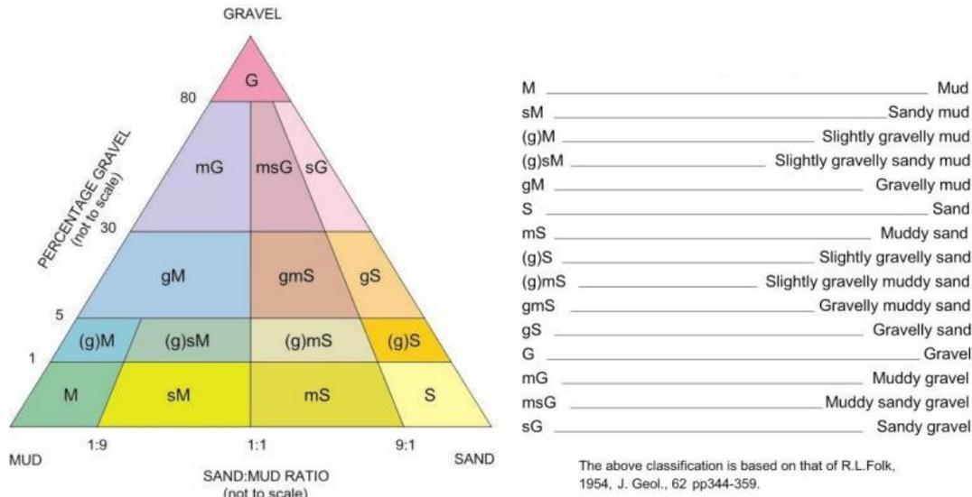
**Figure 6 Folk classification of seabed sediments**
