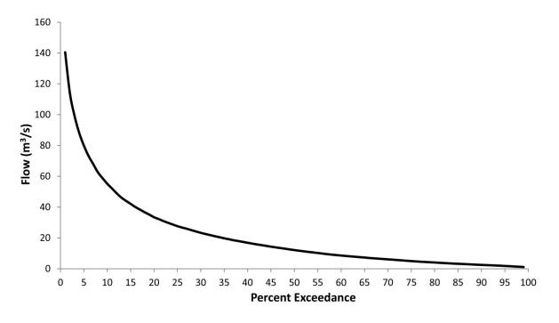
Figure 1.2. A flow duration curve for the River Tamar at Gunnislake gauging station (station number 47001) based upon long-term gauging data (1956 – 1990).
